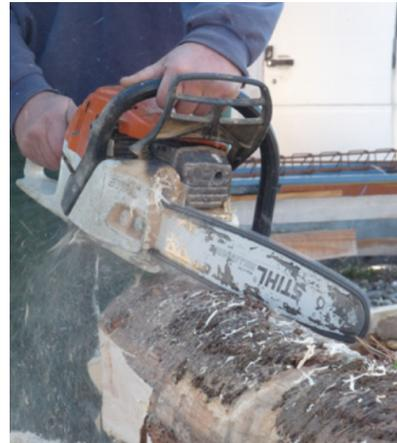
*Figure 8: Decoupe vertical = plus simple*
